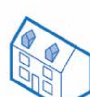
Loft conversion incorporating gable dormers.
