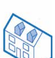
Loft conversion incorporating gable dormers which are out of scale.
