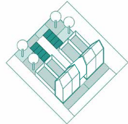
Figure 115: Diagram showing rear parking courtyard
