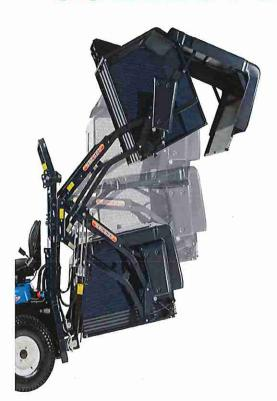
To help make disposing of grass cuttings easy the **SXG323+** and **SXG326+** have an hydraulically operated high or low tip collection system which can lift up to a height of 1.97m.
